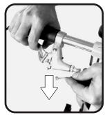
Remove both inner brake cables from both brake levers.(2)
