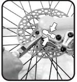
Slide new wire end crimps onto the end of the inner brake cables and apply pressure to secure them.
