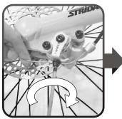
Tighten screw on brake calipers to secure inner brake cables.
