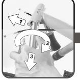
By simply rotating and pulling, you can remove both the handlebars. Note: don't use too much force.
