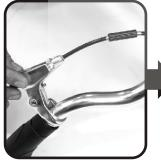
Connect the new inner brake cables to both brake levers.(2)
